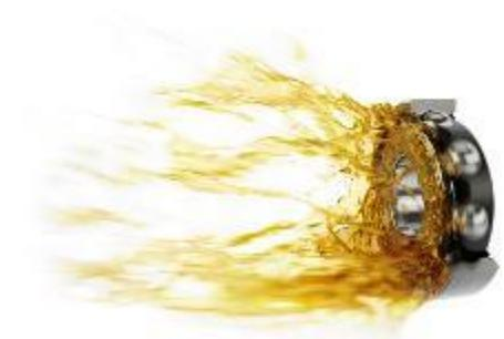
High-performance ball bearing with centrifugal disc: The rotating disc keeps contamination and excessive oil out of the bearing.
