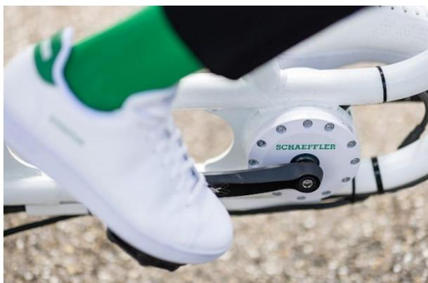
Core component of the system is its pedal generator developed by Schaeffler. It produces constant pedal resistance and provides electricity for the motor in the rear-wheel hub.
